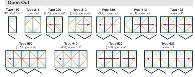
The most common configurations are shown above, but other styles featuring up to seven panes are also possible (please refer to the technical manual). \*No external access or traffic door with this design.
