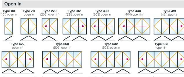
The most common configurations are shown above, but other styles featuring up to seven panes are also possible (please refer to the technical manual). \*No external access or traffic door with this design.
